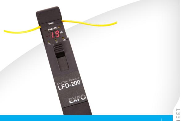
Allows you to detect traffic and measure signals anywhere on singlemode fibers without having to disconnect them.
