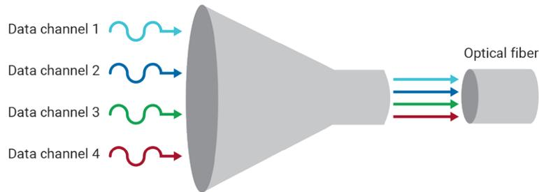
Figure 1. WDM acts as an “optical funnel” using different colors of light (wavelengths) for each signal.
