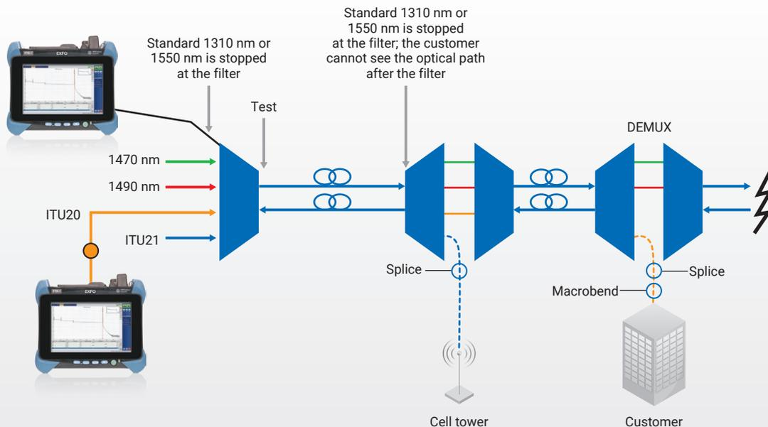
Figure 3. With a CWDM/DWDM OTDR, network service providers can see and validate the complete optical path prior to turning up the service.
